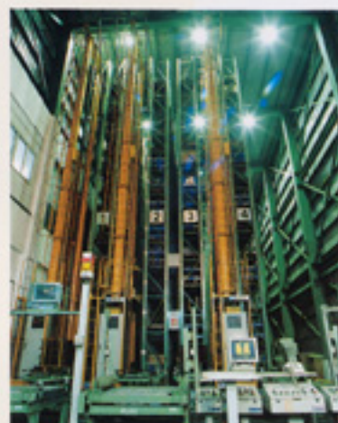
▲ Automatic Storage & Retrieval System
